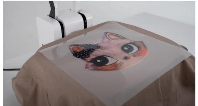
Step 4. Place the baked design with the adhesive powder side facing down on the garment.
