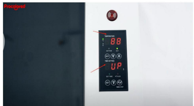
Step 4. The numbers on the top indicate heating temperature, and the numbers on the bottom indicate heating time.
