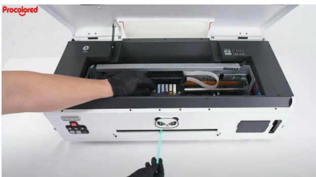
Step 11. Use a cotton swab with warm water to clean the bottom of the print head.
