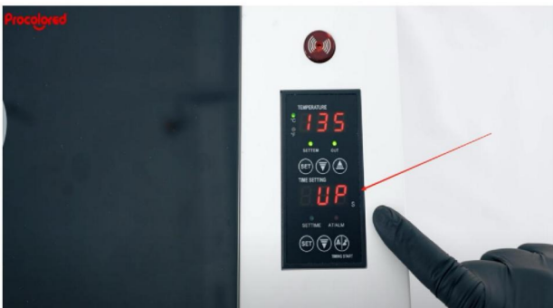
Step 5. Up in the time area means it is still in heating; you can adjust the timing setting.
