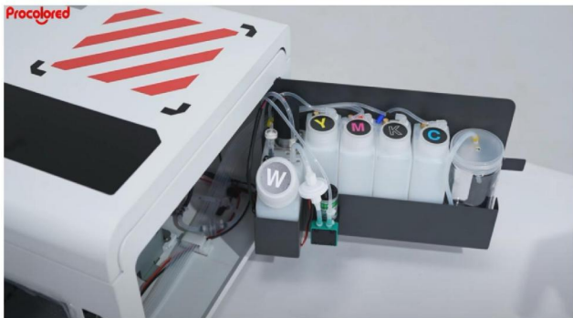
Step 3. Add white ink to W, add yellow ink to Y, add magenta to M, add black ink to K, add cyan to C.
