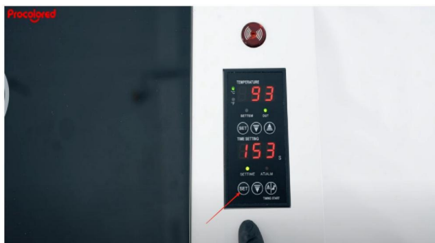
Step 9. Click the set in the time setting area, and adjust the timing for the curing oven.
