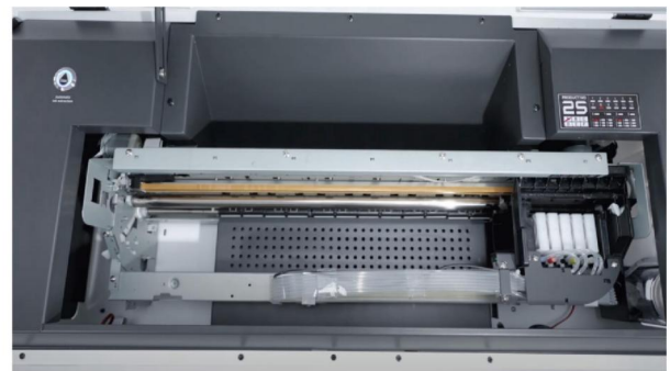
Step 4. The printhead moves while the power button flashes indicating the printer is working properly. (If the printer does not respond contact after-sales support immediately)
