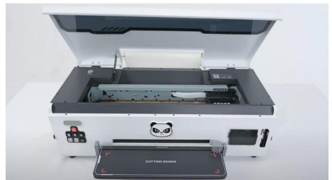
Step 8. Printing is complete when the ink carriage stops and the power button becomes solid blue, No-Ink printing test complete.
