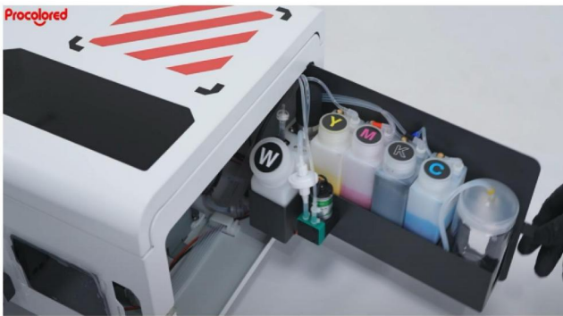
Step 11. Once all inks are added, close the side cover and turn on the printer.
