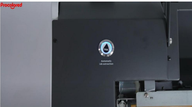
Step 13. After 4-5 seconds, the One-Click Ink Guide Button will start flashing indicating that ink guiding has begun.
