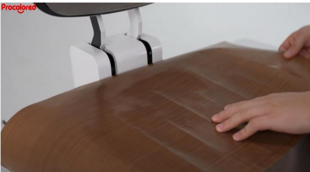
Step 5. Place a teflon sheet over the film.
