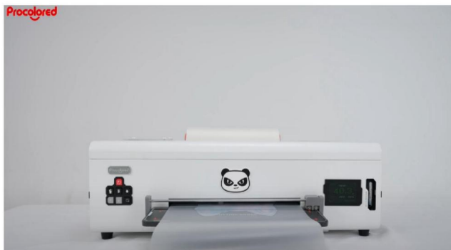
Step 13. Printing begins, the blue power light steady indicates printing is complete.
