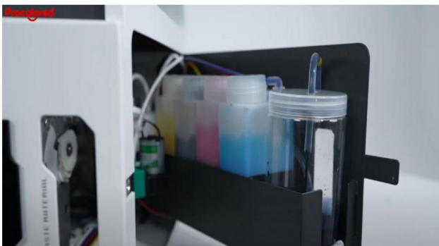
Step 3. And then discharges the waste ink into the container.
