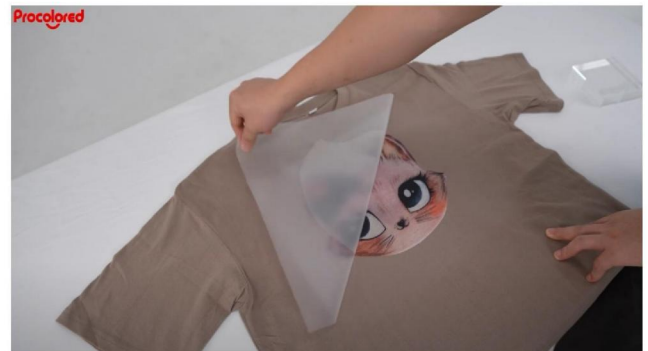
Step 12. Once the design has cooled, slowly peel off the film along the edges of the design.
