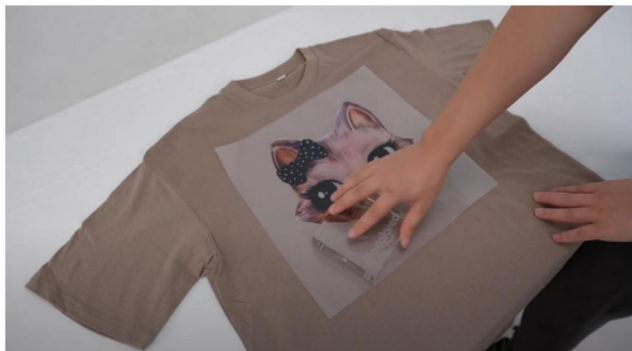
Step 11. It is recommended to use a glass block to cool down.
