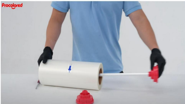
Step 11. Pass the rod through the roll film, make sure the plugs fixed.
