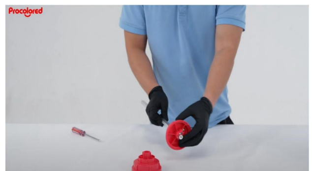
Step 8. Fix the roll film plug on the rod.
