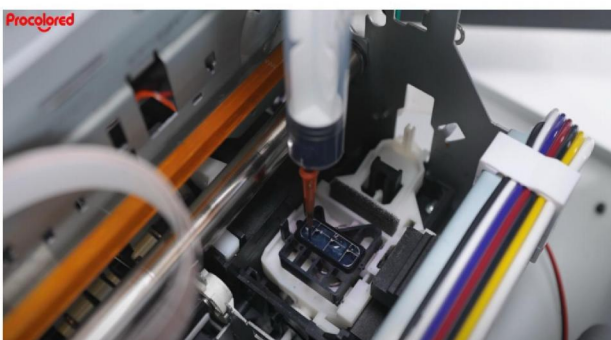
Step 7. Inject warm water into the ink station. Clean the ink station thoroughly. This allows smoother ink extraction.
