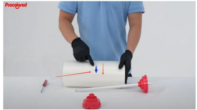
Step 10. put the roll film on the bracket, the arrow on the film should toward the printer.
