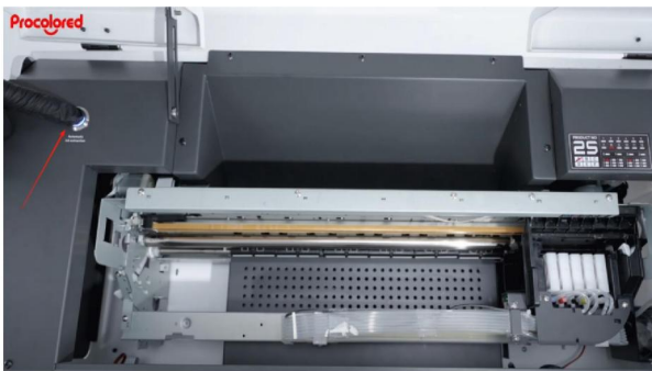
Step 3. This is the One-Click Ink Guide button, press and hold the button for 10s, the ink will be extracted automatically for 45s.
