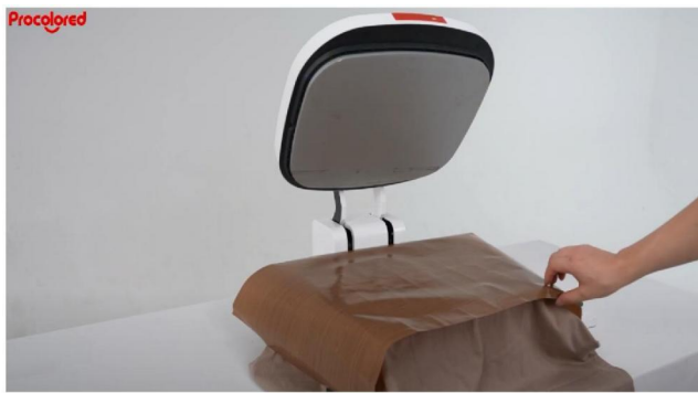
Step 9. Remove the teflon sheet.
