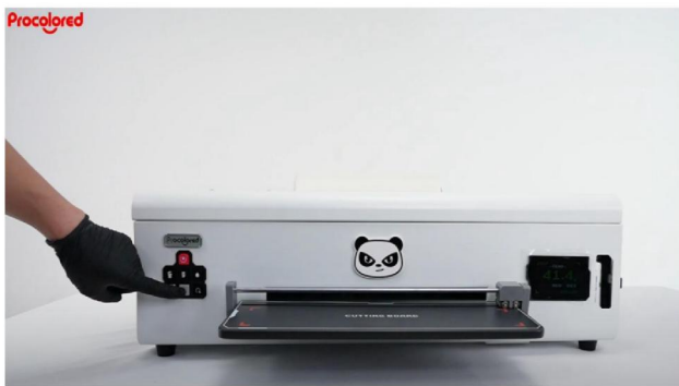
Step 19. Then press the feed button on the front.
