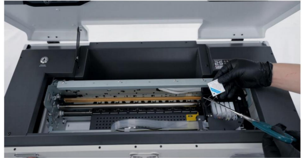
Step 2. Cut off the label and then remove it.
