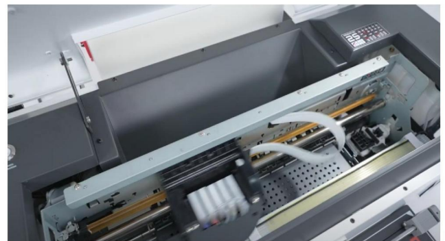
Step 6. The ink carriage starts moving to print. Indicates the printer is operating normally.
