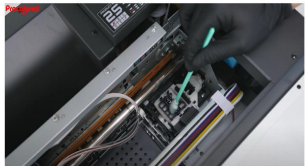
Step 6. Use a cotton swab with warm water to clean the dirty ink in the ink station.
