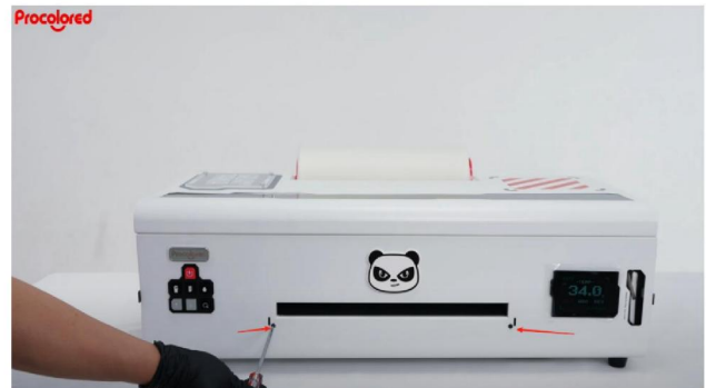
Step 14. Loose the 2 screws on the front, just loose without removing the screws.
