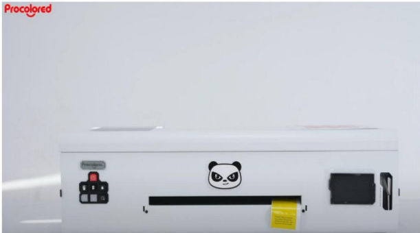
Step 1. Perform printer maintenance every 15 days. This helps reduce the risk of clogged nozzles.
