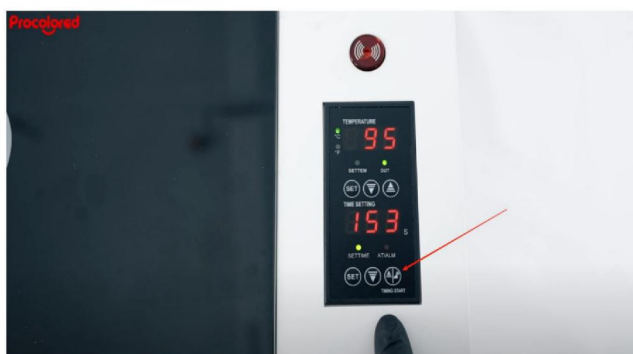
Step 11. Click the up button to increase the baking time.
