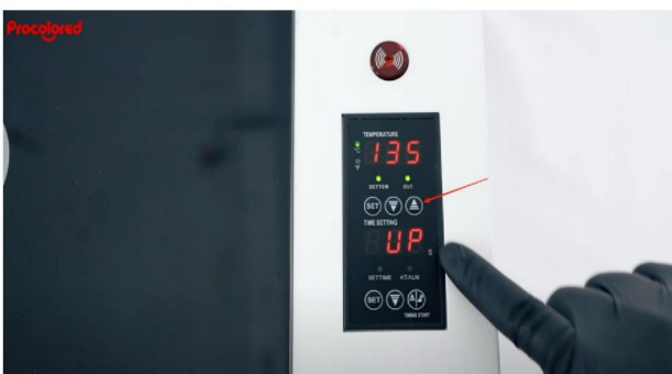
Step 7. The up arrow is used to adjust the temperature setting.
