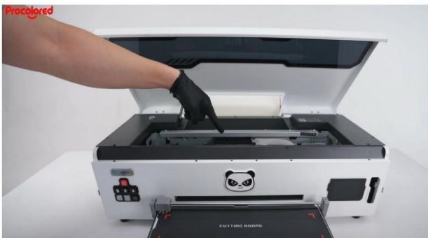
Step 5. Turn off the printer immediately, move the ink carriage to the center.
