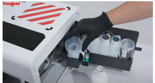
Step 6. Open the white ink bottle and place a funnel on top.
