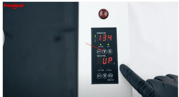
Step 6. The down button is to lower the temperature.
