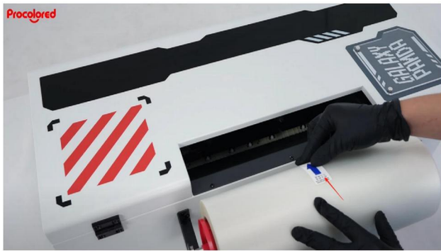
Step 17. The arrow on the film should toward the printer, put inside the printer.
