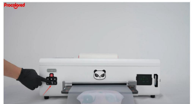
Step 14. After printing is finished long press the paper output button.
