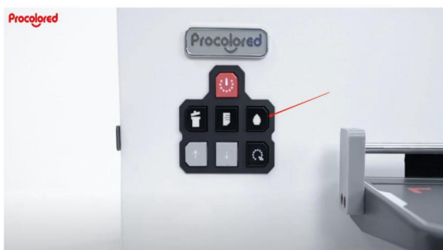
Step 11. Ink Drop Button: Press and hold until the power button flashes to activate printhead cleaning, cleaning is complete when the button stops flashing.
