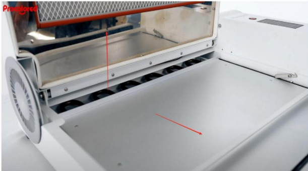
Step 1. Check the oven's exterior, the lid, and the drawer should open easily.
