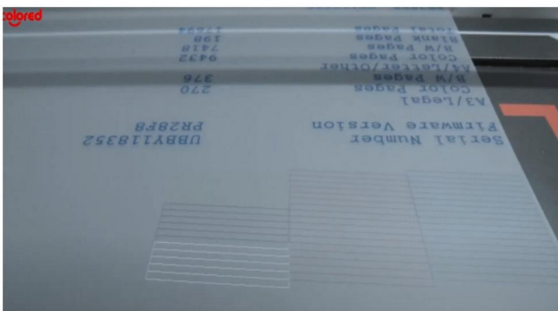
Step 7. If the lines on the test page are complete, it indicates that the print head is good.
