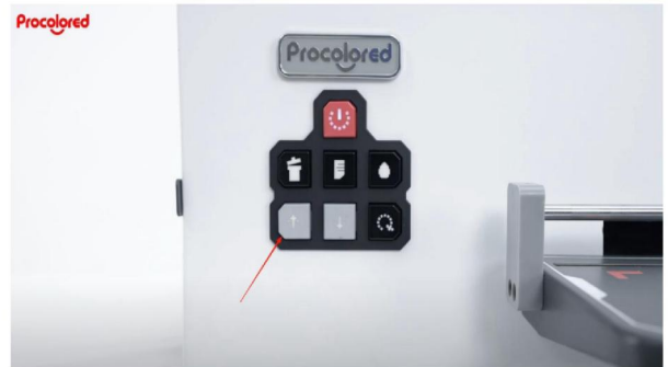
Step 6. Film Rewind Button: press and hold to rewind the film.
