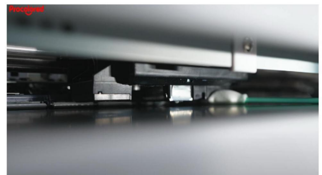
Step 12. Slightly lift the ink carriage; this allows easy insertion of the cotton swab.
