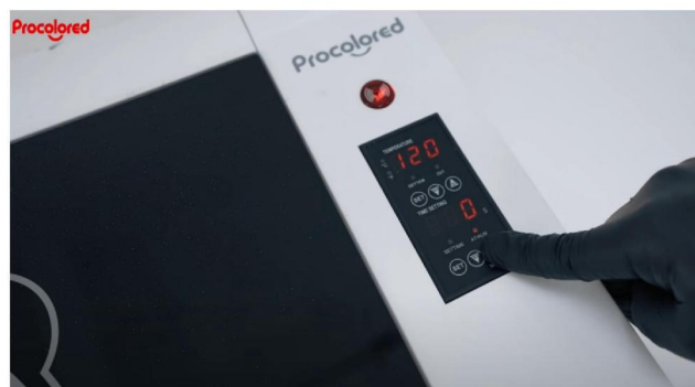
Step 22. An alarm will sound when the countdown ends. Press and hold the Start button to stop the alarm.
