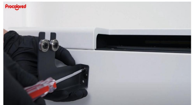
Step 4. Fix the 2 screws for the bracket.
