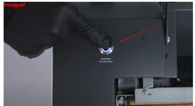
Step 12. After the printer starts, press and hold the One-Click Ink Guide Button for more than 10 seconds.
