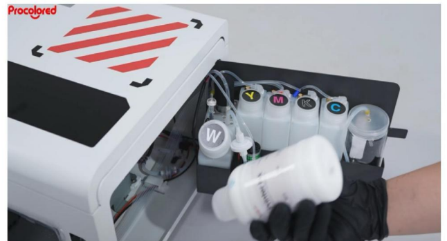
Step 4. Before adding ink, check the label on the bottle and shake it vigorously to make it well mixed.
