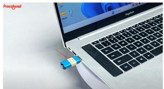
Step 8. Make sure plug in the blue dongle before running the software.
