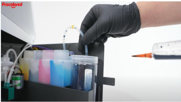
Step 9. Discharge of waste ink into the waste ink container.
