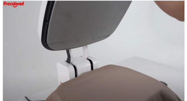
Step 2. Place the garment to be transferred on the heat press and smooth it out.
