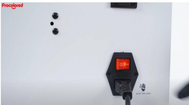
Step 3. After powering on, the ink carriage will start self-check movements.
