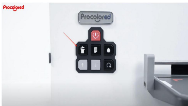
Step 9. Delete Button: press and hold during printing to delete the print task.
