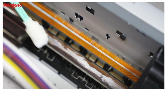
Step 16. Attention: After regular maintenance is completed, it is necessary to run a head cleaning to prevent clogging of the print head.
