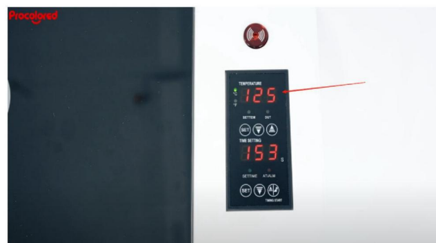
Step 14. When the up change to digital value means heating completed, the oven is ready to use.
