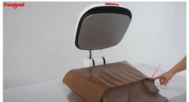
Step 6. Start the heat press and set the temperature to 160 degrees for 35 seconds.
