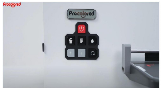
Step 18. Wait until the power button stops flashing this means the cleaning process is finished and you're finished all ink filling task.
