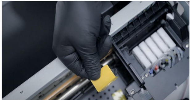
Step 4. Then remove the latches securing the ink carriage. The latches keep the ink carriage in place preventing the carriage from moving during shipping.
