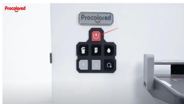
Step 12. Power Button: click to turn the printer on and off.
