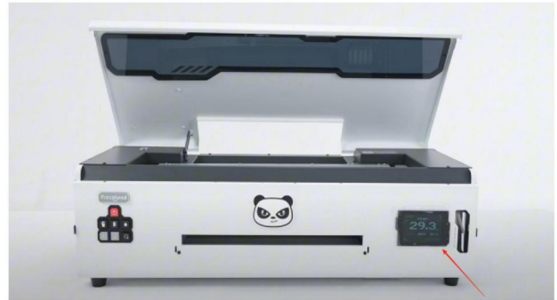
Step 2. The power indicator and temperature panel will light up when startup complete.
