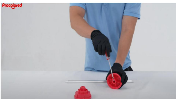
Step 7. Loosen the screw on the roll film plugs.
