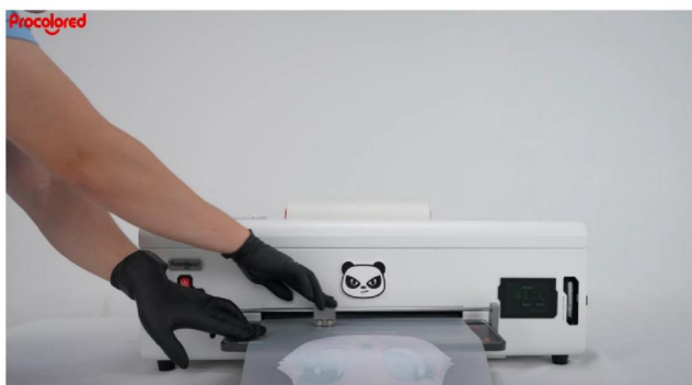
Step 15. Cut the film paper with a cutter. (Note: the white ink has not cured yet, do not touch the design.)
