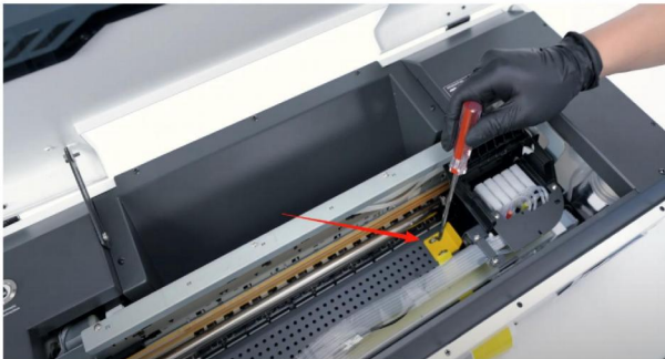
Step 3. Use a screwdriver to unscrew the screws holding the ink carriage latches.
