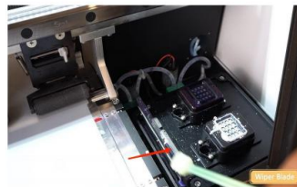
Step 14. Clean the wiper blade at left side first, do proceed the cleaning gently.
