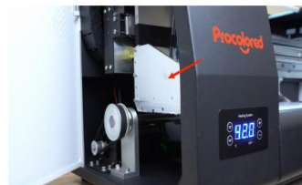
Step 19. Now we open the side door and the arrow points to where the print head is.
