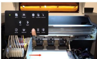
Step 9. Remember to press base points button to set the print head assembly back to right side.
