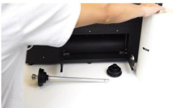
Step 17. Now we're about to insert the film roll.
