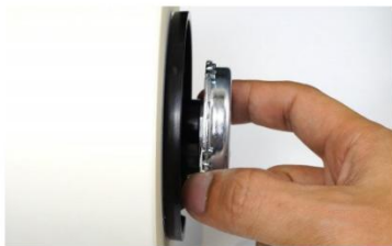
Step 23. Adjusting the film roll and plastic holders position - the film roll better be placed in the middle or right side of the roller bar. Then insert the bar holder taken from the right bracket on the right side of the roller bar.
