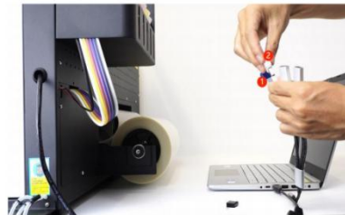
Step 4. Insert the two USB devices. ① The blue one is a RIP dongle, you'll need it every time you use the RIP software. ②The white one is a regular USB thumb drive stored with guidance videos and printer software.
