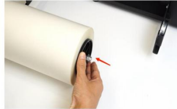
Step 22. Insert the plastic holder of the other end and push it in.
