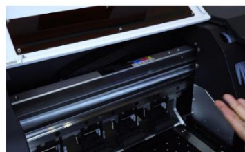
Step 4. The metal plates secure the drive belt during transportation but if you forgot to remove them before the machine is powered on, the drive belt could become deformed.
