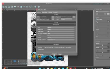
Step 4. Choose Automatic print after RIP and click print to initiate the task.
