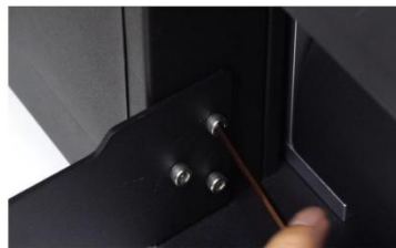
Step 14. Fasten the screws. The DTF film roller is quite heavy, so the screws of the bracket should be fasten well.
