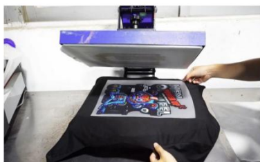
Step 17. When the preheating is done, apply the printing sheet on fabric. Remember to double confirm the printing placement.
