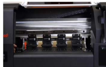
Step 34. When the lever is pulled up, the film advance array rollers will raise.
