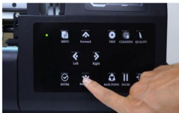
Step 52. Press the "Forward" and the "Backward" buttons to check the film feeding situation.
