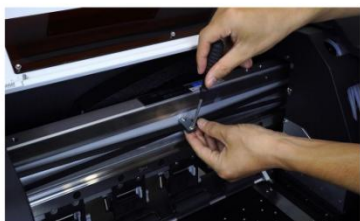
Step 3. Use screw driver to remove the metal fixing plates on the drive belt.
