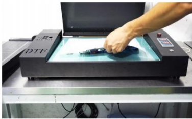
Step 11. Set the temperature at 120 degrees Celsius and the countdown timer to 180 seconds. Then gently put the film on the oven pad. [color side down]
