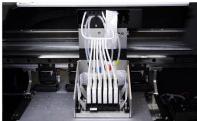
Step 5. Here we can see all the ink tubes and cartridges.
