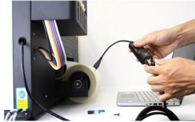
Step 2. Plug the printer cable into the USB adapter for fast data transfer. If your WAN port can reach the speed of 1 Gigabit per second, you don't need this USB adapter.
