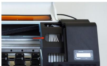
Step 51. As soon as the printer is powered on, the white ink circulation system will start automatically.
