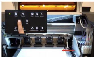
Step 7. When we finish cleaning the left part, press left button on the control panel to move the print head assembly.
