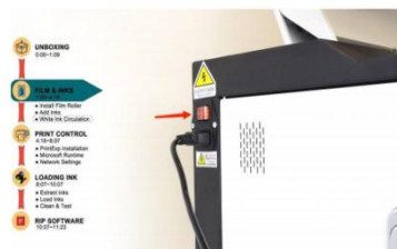
Step 50. Power on the printer. [the button situation in this picture means "off"]
