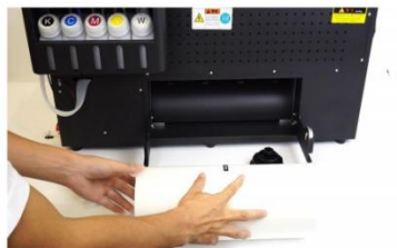
Step 19. The arrow sign on film should point to the printer.
