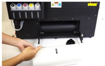
Step 18. Before inserting the roller bar through the DTF film roll, pay attention to the direction of the film leading edge. Only the outer surface of the DTF film is printable.
