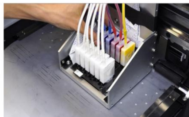
Step 10. Gently put the ink cartridges back when the extracting work is done.
