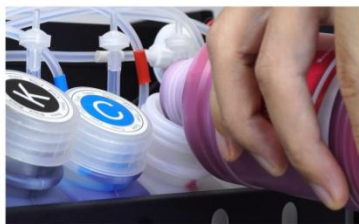
Step 43. Fill the ink in sequence. If you pour the wrong ink, you need to empty the ink from the tank with syringe and ink pumping tube.
