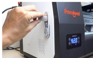
Step 18. Then hold the upper handle and rotate it to the left.
