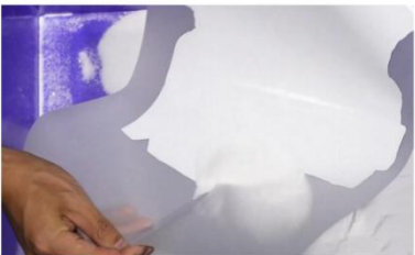
Step 9. Cool the printing sheet for 1 minute, then spread adhesive powder evenly on the white side of printing.
