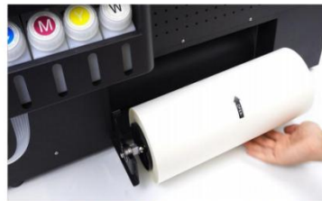
Step 26. Make sure the film rollers stays stable on the brackets.
