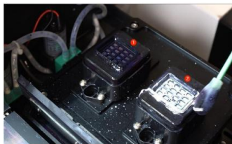
Step 15. Then we go on cleaning the two cappings. It's obvious that capping ① of color ink is more easily cleaned; capping ② is for white ink, on which residues will be more and be harder to be wiped off.
