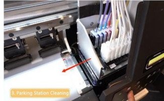
Step 12. Parking station also needs regular cleaning and maintenance. Press left button to move the print head assembly to the left.
