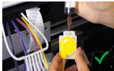
Step 8. Take off only one cartridge at a time and turn it upward to extract 5 to 10 millimeters of ink until the cartridge is free of air.
