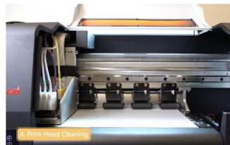
Step 16. Now let the print head assembly remains on the left, we're going to clean the print head bottom.
