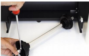
Step 15. Loose the screws on the two ends of the roller bar.
