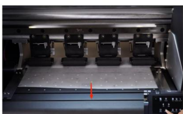
Step 53. Make sure the film sheet can pass through the printing platform smoothly.
