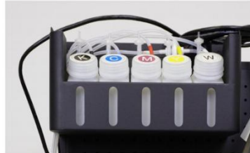
Step 42. K refers to black ink, C refers to cyan ink, M refers to magenta ink, Y refers to yellow ink and W refers to white ink.
