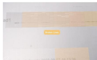
Step 4. Lines with gaps indicate there may be nozzle blockage or ink supply issues. Yet this is common to see, since when a printer is just initiated, its nozzle needs to do some spraying first to get itself unobstructed.
