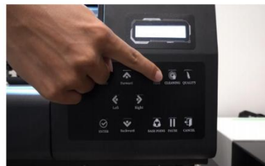
Step 8. When the cleaning is finished, press test button again.
