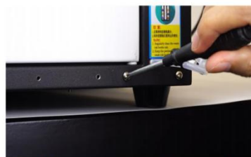
Step 44. Now we're going to install the waste ink bottle. First remove the screws.
