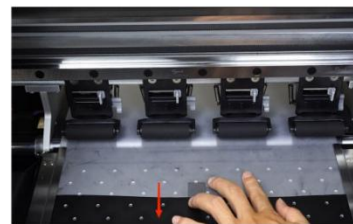
Step 36. Guide the film sheet to go under the 2 metal plates on the printing platform.
