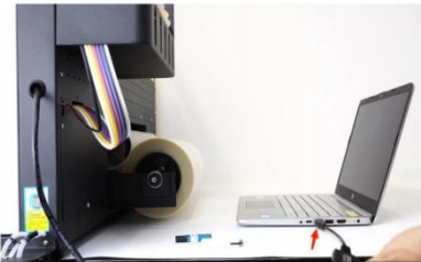
Step 3. Connect the USB adapter with your computer. (Procolored software only works on Windows computers)
