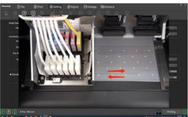
Step 19. During the checking process, the print head assembly will move back and forth and print a testing chart.
