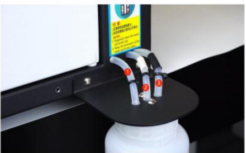
Step 47. ①The one without label is for waste ink that dropped off from the print-head parking position ②the one with white label is for white waste ink ③the one with black label is for inks of all the other colors.
