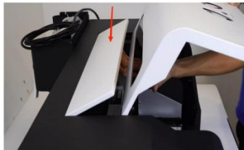
Step 2. And at the same time open the top cover and move both of them to the maximum angle.
