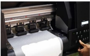
Step 7. Press forward button on the control panel to load more spare film forward.
