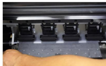
Step 37. Pull down the lever now to put the film advance array rollers down.
