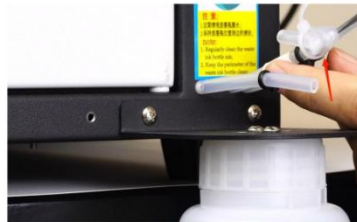
Step 46. Cut the tube tie. The printer comes with 3 waste ink tubes.
