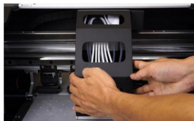
Step 4. Remove the black cover of the print-head assembly.
