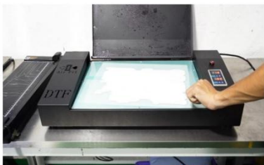
Step 13. When curing time is up, gently fetch the cured printing. We highly recommend to use a suction cup to fetch the cured printing film, since the oven pad and film might be really hot.
