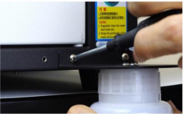
Step 45. Place the printer at the edge of the table, put the waste ink bottle in place and fasten the bottom side rail screws.
