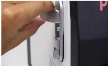
Step 31. Rotate the upper handle to the left.
