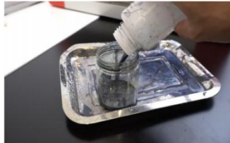
Step 2. Pour out the waste ink, ink waste bottle should be emptied regularly.
