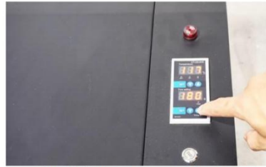
Step 12. Press start button to initiate the curing.
