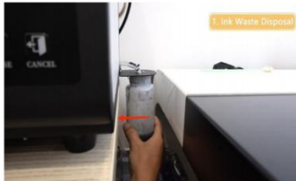
Step 1. Rotate clockwise to remove the ink bottle and remember to hold a tray beneath in case of any accidental ink drops.
