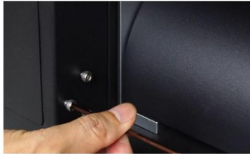
Step 11. Loose the screws on the left side first.
