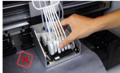
Step 6. Don't take off all the ink cartridges at the same time. Some ink cartridges are interconnected, air will enter other ink tubes.
