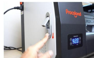
Step 17. Slide the bottom button down, then the upper handle will pop out automatically.
