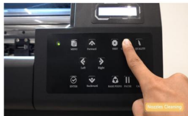
Step 5. When there's gaps in test chart, press cleaning button to start nozzle cleaning process.
