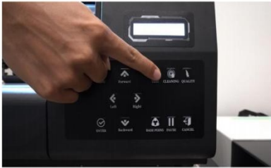
Step 1. Press test button on the control panel to initiate nozzle checking function.
