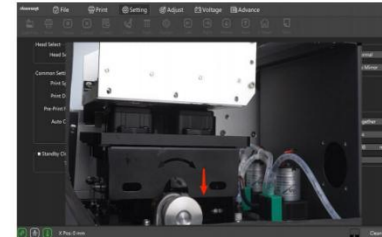
Step 16. During the cleaning process, the capping station will automatically press down.
