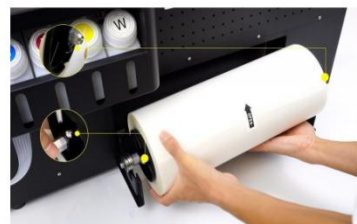
Step 24. Remember to fasten the screws on both plastic holders before loading the film roller.
