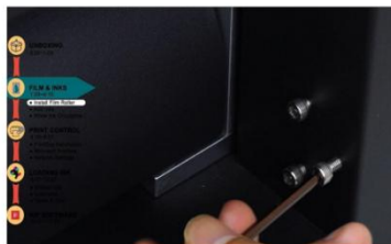
Step 6. Use an Allen key to remove the preinstalled screws of the right bracket position.
