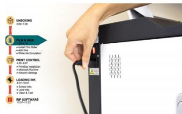
Step 48. Plug the printer cable in.
