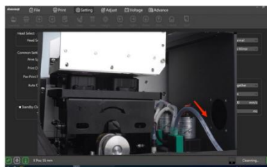
Step 17. And the waste ink will flow through the tube. The cleaning takes about one and a half minutes to finish.
