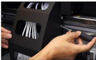
Step 3. Undo the screws at both sides.
