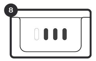
During calibration, the lights will progressively light up white. Once successful, the first light will flash white, before staying on to indicate it is now in Normal Mode.
