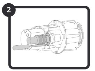
Fasten the flexible drain tube at the bottom of the Separator, making sure it is watertight. (Bolts might squeak when fastening, this is normal.)
