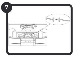
Press the Collection Center up against the Separator's foam ring. Then, reach in through the opening at the top and connect the data cable.
