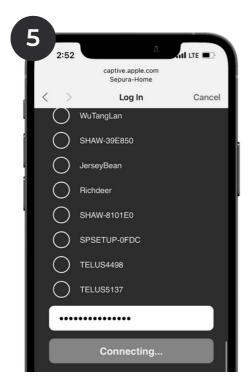
Once on the splash page, hit the "Scan Wi-Fi" button, this will display a list of all available networks. Select your home Wi-Fi (note that only 2.4GHz is accepted), scroll down and enter your Wi-Fi password and hit Connect.
