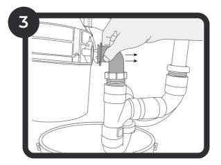
Disconnect the drain pipe from the rest of the plumbing (there might be some water that drips down at this stage, so have a bucket handy).
