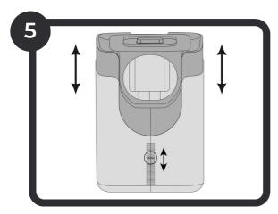
Now, grab Sepura's Collection Center, remove the bucket and lid inside, and slide into place with the door facing you. Adjust its height by sliding the top compartment until the Separator component fits inside the back opening.
