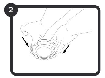
Roll up the plumber's putty into a thin, long roll and apply around the bottom side of the flange ring. Center the flange in your sink and press down firmly to create a seal.
