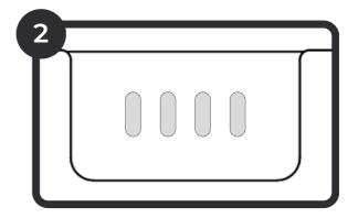
Sepura will then create an Access Point to connect to Wi-Fi. Its progress will be shown by the lights loading in green. Once the Access Point is ready, the lights will blink slowly green.
