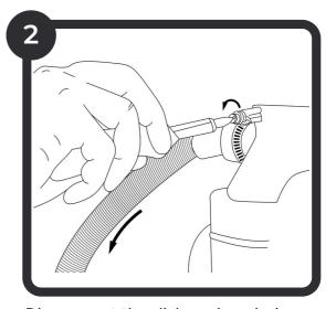
Disconnect the dishwasher drain tube (if installed).
