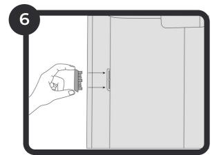
Once a height is reached where the Separator can fit through the back opening of the Collection Center freely, lock the height in place with the side clips.
