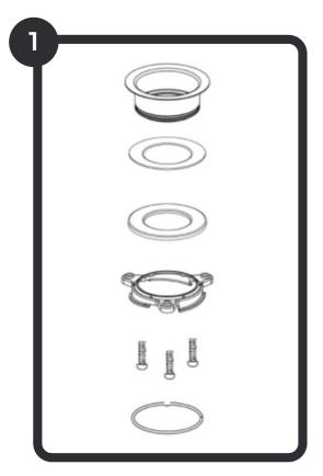
You can now grab the 3-bolt sink mount from the box. Separate the flange by loosening the three bolts and removing the snap ring.
