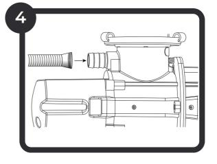
(OPTIONAL) If you have a dishwasher drain, connect this to the Separator's dishwasher drain inlet. Make sure the plug was knocked out in step 1.
