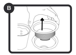
Remove the flange by pushing up underneath it and then removing it from inside the sink. Make sure any food waste and glue residue is wiped clean and dried before continuing.
