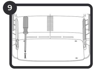
Secure the Collection Center into the baseboard with the 4 wood screws left.
