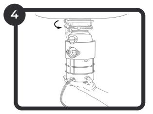
Twist the sink mount ring attached to free the garbage disposal (if stuck, use your screwdriver inside the loops to create leverage). The disposal unit is heavy, so prepare for that to avoid damage to your plumbing.
