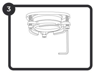
Go underneath your sink and reassemble the parts of the mount as they were before. Use the snap ring to lock them into place. Tighten the 3 bolts by increments like a car tire to create an even space all around.
