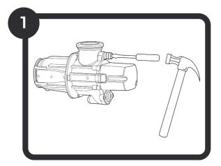
(OPTIONAL) Grab Sepura's Separator component and if you have a dishwasher drain, knock out the plug with your hammer and screwdriver.
