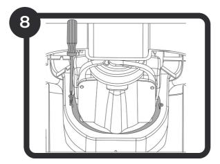
Make sure the Collection Center is pressed up against the Separator's foam ring to create an air-tight seal, then use the 2 small screws provided to fasten the two together.
