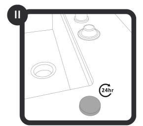
Press the button, adhesive side down, firmly into place. Wait 24 hours before wetting the area again.
