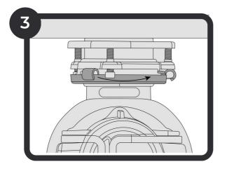
Position the Separator under your sink with the valve door and latch facing you. Connect it to your sink by twisting the bottom ring onto the 3-bolt sink mount. Make sure the Separator's gasket is in place (in between the sink mount and its drain opening) and to tighten the mount's ring all the way up to the notch, otherwise leaking can occur. Then, connect the flexible drain tube to your plumbing, making sure it is watertight.
