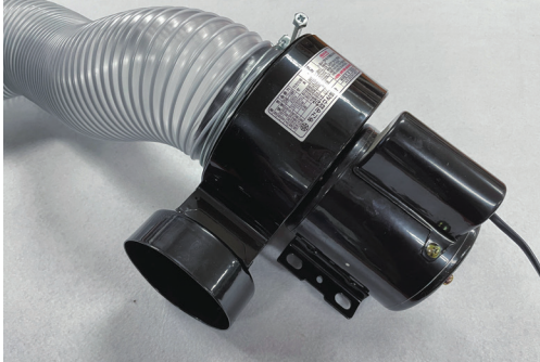
*Required Ring blower spec* Diameter 4", over 170CFM
