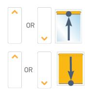
Step 4: PRESS & HOLD the MY/STOP button until the shade jogs, then release. Check the new limit.
