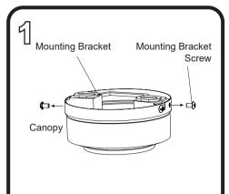
Loosen all four mounting bracket screws and completely remove the two screws from the round holes in the canopy. Save the screws for later. Remove the canopy from the mounting bracket.
