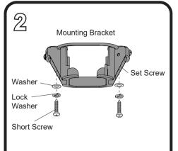
Use 2 short screws along with washer and lock washer to secure the mounting bracket to ceiling joists. Then, loosen but do not remove two set screws on each side of the mounting bracket.
