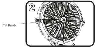
3. Use adjustment handle located on bottom of fan to change the direction of airflow from left to right
