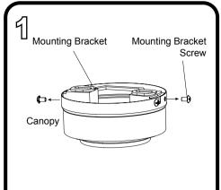
Loosen all four mounting bracket screws and completely remove the two screws from the round holes in the canopy. Save the screws for later. Remove the canopy from the mounting
