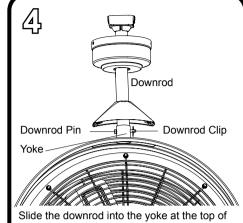
the fan and turn clockwise until the holes in the downrod align with the holes in the yoke. Then reinstall the downrod pin and downrod
