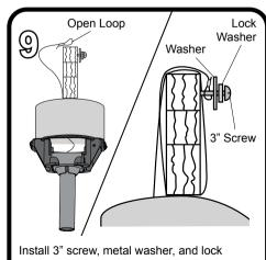
washer partly into the side of the brace installed in the ceiling. Then lift the braided cable up and over the ceiling brace and place the open loop of the braided cable around the secondary support screw. Tighten 3" screw.
