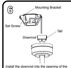
mounting bracket. Tabs on downrod should face the sides of the mounting bracket to engage the slots inside the mounting bracket. Retighten the two set screws to secure.
