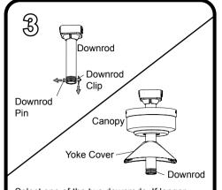
Select one of the two downrods. If longer downrod is needed, see page 2. Then, remove the downrod clip and downrod pin from the downrod. Insert the downrod through the canopy and yoke cover.
