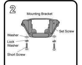
Use 2 short screws along with washer and lock washer to secure the mounting bracket to ceiling joists. Then, loosen but do not remove two set screws on each side of the mounting
