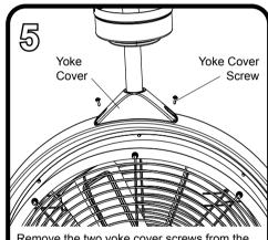
Remove the two yoke cover screws from the top of the fan. Use the two yoke cover screws to secure the yoke cover to the top of the fan assembly. Then, lower the yoke cover to rest on top of fan assembly.
