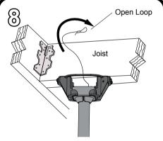
Feed the loop of the braided cable, preassembled to the downrod, up through ceiling and around the ceiling joist. Important: The braided cable must make a complete circle around the support brace. Note: Joist may need to be accessed from attic.
