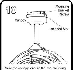
Raise the canopy, ensure the two mounting bracket screws are aligned with the J-shaped slots in the canopy. Then turn the canopy in a clockwise direction until the mounting bracket screws are completely engaged in the J-shaped slots.
