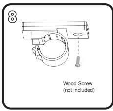
(Optional) Cord clips have a round hole to accommodate a wood screw (sold separately) as an option to the taping method.
