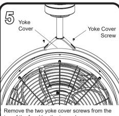
top of the fan. Use the two yoke cover screws to secure the yoke cover to the top of the fan assembly. Then, lower the yoke cover to rest on top of fan assembly.
