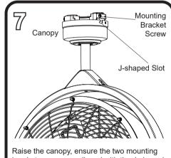
bracket screws are aligned with the J-shaped slots in the canopy. Then turn the canopy in a clockwise direction until the mounting bracket screws are completely engaged in the
