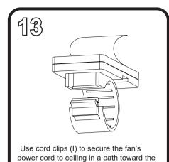
power outlet. Peel the backing off of the
