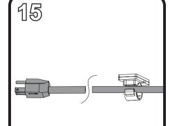
Secure each cord clip (I) to the ceiling. Then insert the cord into each clip and press the clip closed to secure the cord. Note: Leave adequate slack near the fan to allow fan to swivel and/or tilt.
