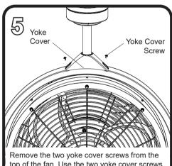
top of the fan. Use the two yoke cover screws to secure the yoke cover to the top of the fan assembly. Then, lower the yoke cover to rest on top of fan assembly.
