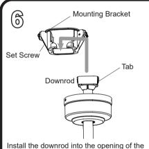
mounting bracket. Tabs on downrod should face the sides of the mounting bracket to engage the slots inside the mounting bracket. Retighten the two set screws to secure.
