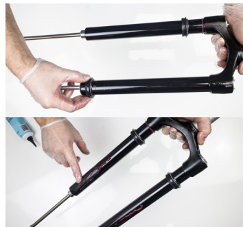
17. Slide NEW wiper seals & soaked foam rings onto the Inner stanchion legs and lightly grease.
