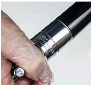
12. Re-tighten in the inner stanchions. 18Nm
