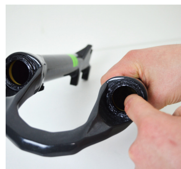
18. Apply grease over the foam rings.
