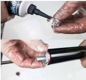
11. Grease the thread on the bottom alloy air cap
