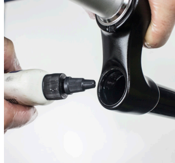
14. Add approx. 6ml of 5W fork oil down the Air side inner stanchion.
