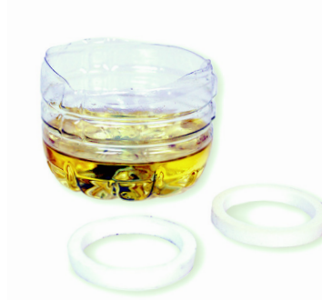
16. Soak each NEW foam ring in 80W gearbox oil until saturated.
