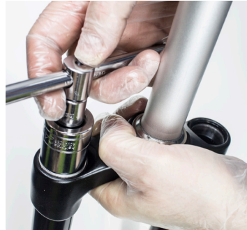
15. Re-fit the alloy air valve seal top cap using 24mm socket. 18Nm
