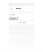
3. Choose "Up limit", tap "open" or "close" to the desired Up limit position, then "pause", tap "Save limit", the Up limit setting done. Motor runs downwards automatically, tap "pause" when it reaches the desired Lower limit position.
