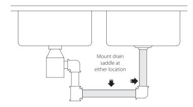
2. Next, align and install the drain saddle clip with the tubing connection port onto the black sponge. This will cushion any gap between the saddle and the pipe. Make sure the hole on the sponge is thoroughly punched out, and is aligned to the hole on the saddle to complete the installation.
