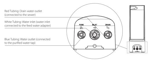
Illustration of the quick connect ports
