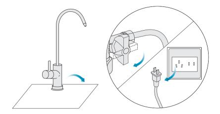
2. Unscrew the existing filter cartridge counterclockwise and relieve the pressure.
