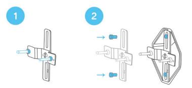
Insert fixture long screws and nuts into the Bracket as shown
