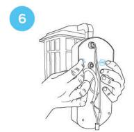
Holding the light fixture with both hands, align the two fixture long screws into the light fixture screw-posts.
