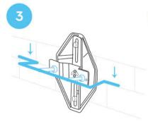
Use screw length indicator to adjust the length of the two long screws from the wall, then tighten the two nuts.
