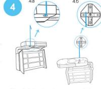
Use holding hook to suspend the light and free your hands for wiring. Connect the bottom of the hook (Square) to the right screw pole, than hang the top of the hook on the mounting bracket.
