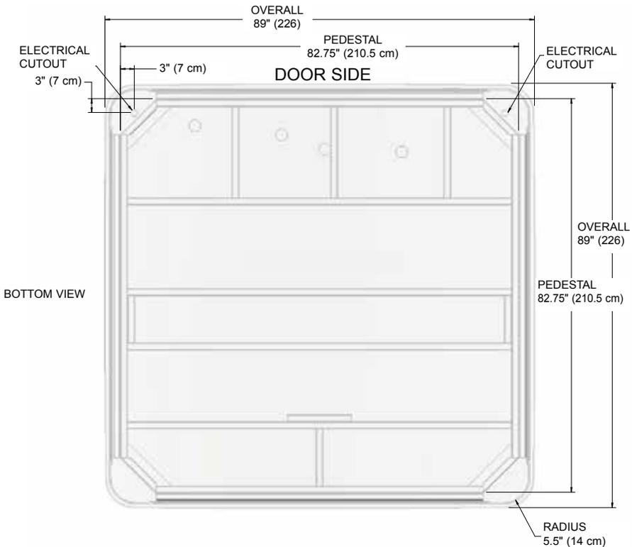
**NOTE: WATKINS WELLNESS** requires that the **MAKENA** and **SALINA** be installed on a minimum 4" (10 cm) thick reinforced concrete pad or structurally sound deck able to support the "dead weight" found in the chart on the back page.
