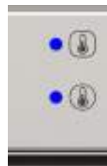
Fig. 12 Indicator light for chamber and boiler heaters
