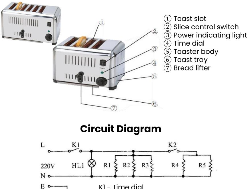
K1 - Time dial K2 - Slice control switch HL1 - Power indicating light R1~R5 - The electric thermal plate
