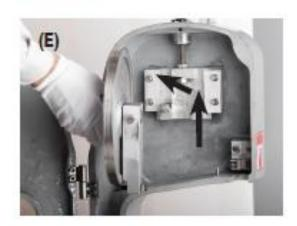
F. Please use low pressure squirt gun to spray the interior minced meat, then reinstallment in order. A Electrical parts(as exterior control knob,switch....) can't be directly sprayed by squirt gun.
