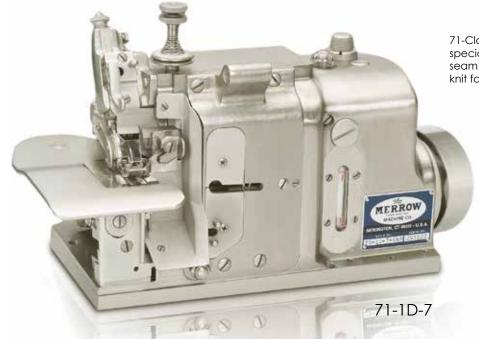
71-Class cams have specially-milled grooves to seam at 4000 rpm on knit fabric.
