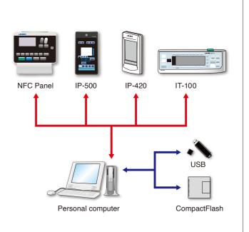
The sewing machine can be paired with equipment which supports NFC (Near Field Communication)
