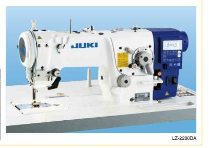
High-speed, 1-needle, Lockstitch, Zigzag Stitching Machine (with standard / 3-step zigzag stitching pattern changeover function)
