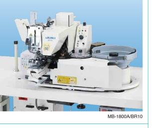
Single-thread, Chainstitch, Button Sewing Machine (thread-fray-prevention ON/OFF changeover mechanism)
