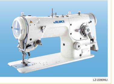
High-speed, Cylinder-bed, 1-needle, Lockstitch, Zigzag Stitching Machine (with standard / 3-step zigzag stitching pattern changeover function)
