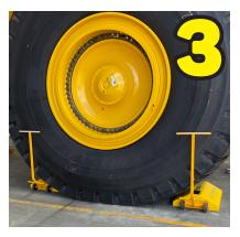
When chocks on both sides of the wheel are in position correctly, the truck is secured.
