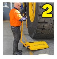
Lift the chock onto its front wheel and bring close to the tire. Bring the back of the chock around into position.
