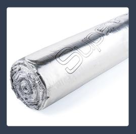
Cut using the most appropriate tool for the thickness of the SuperFOIL product you are using, staple in place over the pitched roof timber rafters, from the ridge to the eaves, using the correct size galvanized or stainless-steel staples at 300mm intervals.
