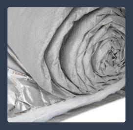
Cut using the most appropriate tool for the thickness of the SuperFOIL product you are using, staple in place over the pitched roof timber rafters, from the eaves to the ridge, using the correct size galvanized or stainless-steel staples at 300mm intervals.
