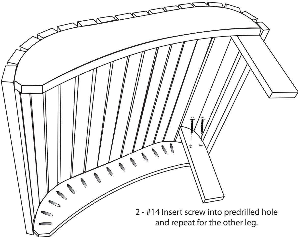
2 - #14 Insert screw into predrilled hole
