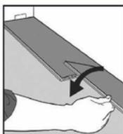
**Step 4** - At the end of the first row, leave a ¼" gap, to the wall and measure the length of the last plank and cut it off.
