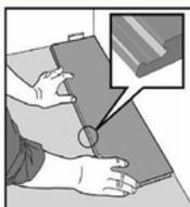
**Step 2** - Second plank, first row. Drop this plank gently to the narrow end of the first plank.
