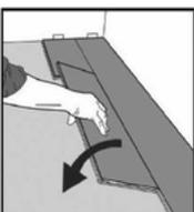
**Step 9** - Press or tap along the narrow end of the installed panel.
