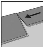
**Step 3** - During the drop down, make sure the planks are tight against each other. Press or tap at the narrow end just installed. Use a rubber mallet if necessary to ensure an engaged lock on the short side.
