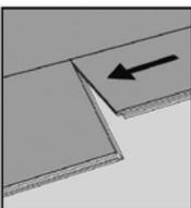
**Step 8** - Click the plank to the narrow end of the previous panel. During the fold down, make sure the planks are tight against each other.
