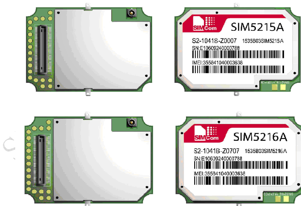
Figure 40: Top and bottom view of SIM5215/SIM5216
