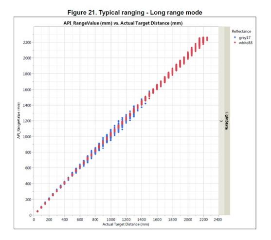
Depending on ambient lighting and distance, you'll get 3 to 12% ranging accuracy - better lighting and shiny surfaces will give you best results. Some experimentation will be necessary since if the object absorbs the laser light you won't get good readings.
