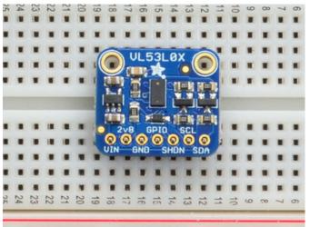
Place the Breakout board on top so the shorter ends of the pins line up though all the pads
