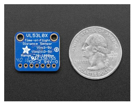
Communicating to the sensor is done over I2C with an API written by ST, so its not too hard to port it to your favorite microcontroller. We've written a wrapper library for Arduino so you can use it with any of your Arduino-compatible boards.
