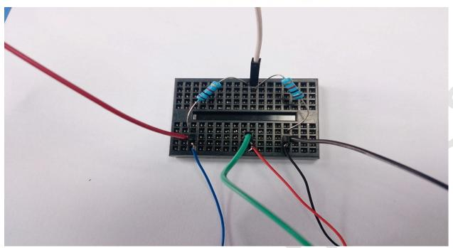
Connect Load Cell Half bridge 50KG with Weight Scales Analog-to-Digital Converter (ADC) 24-bit and arduino
