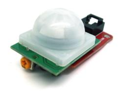
**Sensitivity range:** up to 7 meters 110 degrees x 70 degrees detection range.
