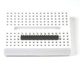
Prepare the header strip Cut the supplied header strip to length and insert it longpins-down in your breadboard to hold it for soldering.
