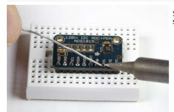
Solder! Solder each pin for a good electrical connection.
