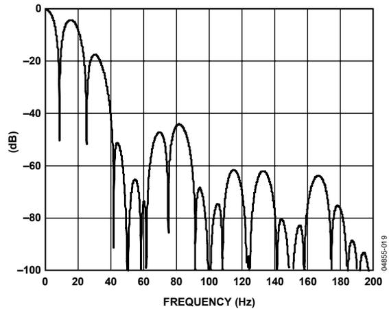
Figure 14. Filter Profile with Update Rate = 16.7 Hz
