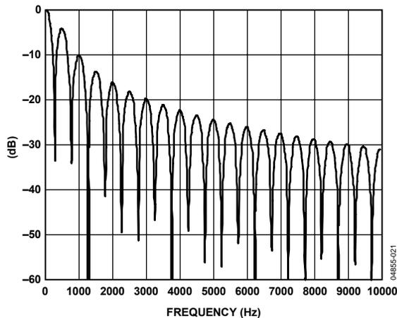
Figure 16. Filter Response at 470 Hz Update Rate
