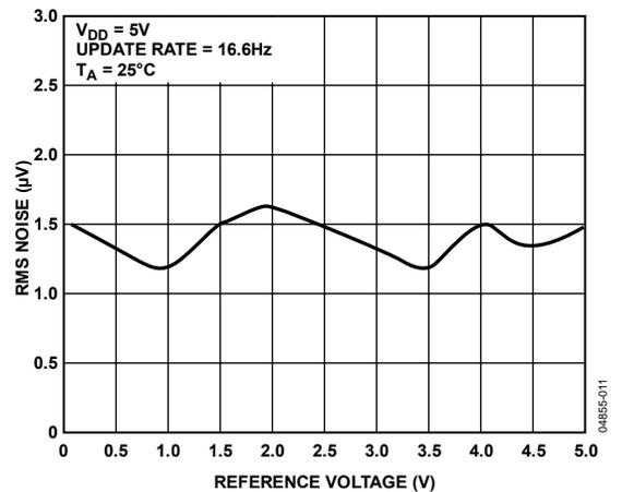
Figure 11. RMS Noise vs. Reference Voltage (Gain = 1)
