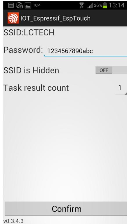
(3)When app creates IP (192.168.0.189 for example ) successfully ,ESP-01 module connects router already .It will remember account and password .And it will connect router automatically when go into mode 2 next time .
