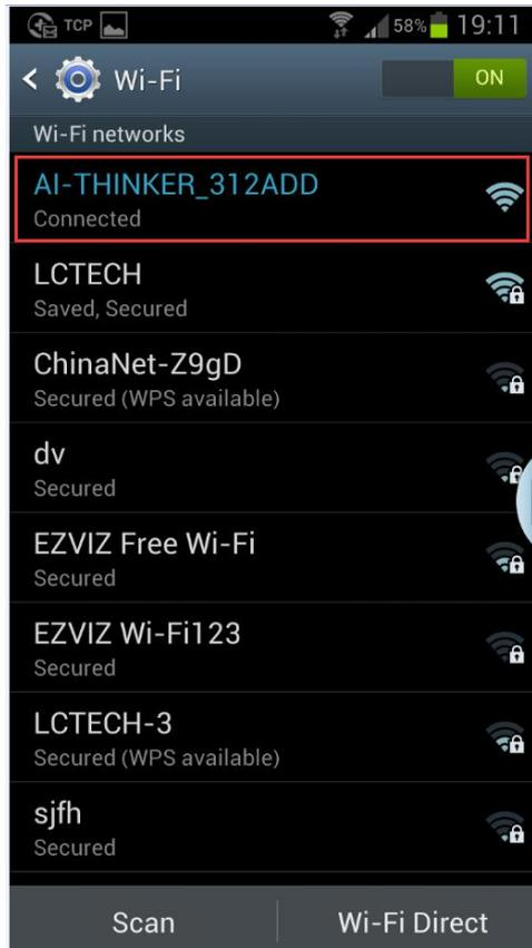
(3)log in app “EasyTCP\_20 “,CLICK “CONNECT”,input IP 192.168.4.1 ,port 8080 ,then connect .The green LED will be 2s slow blinking to always on .Click gray block to control the relay now .
