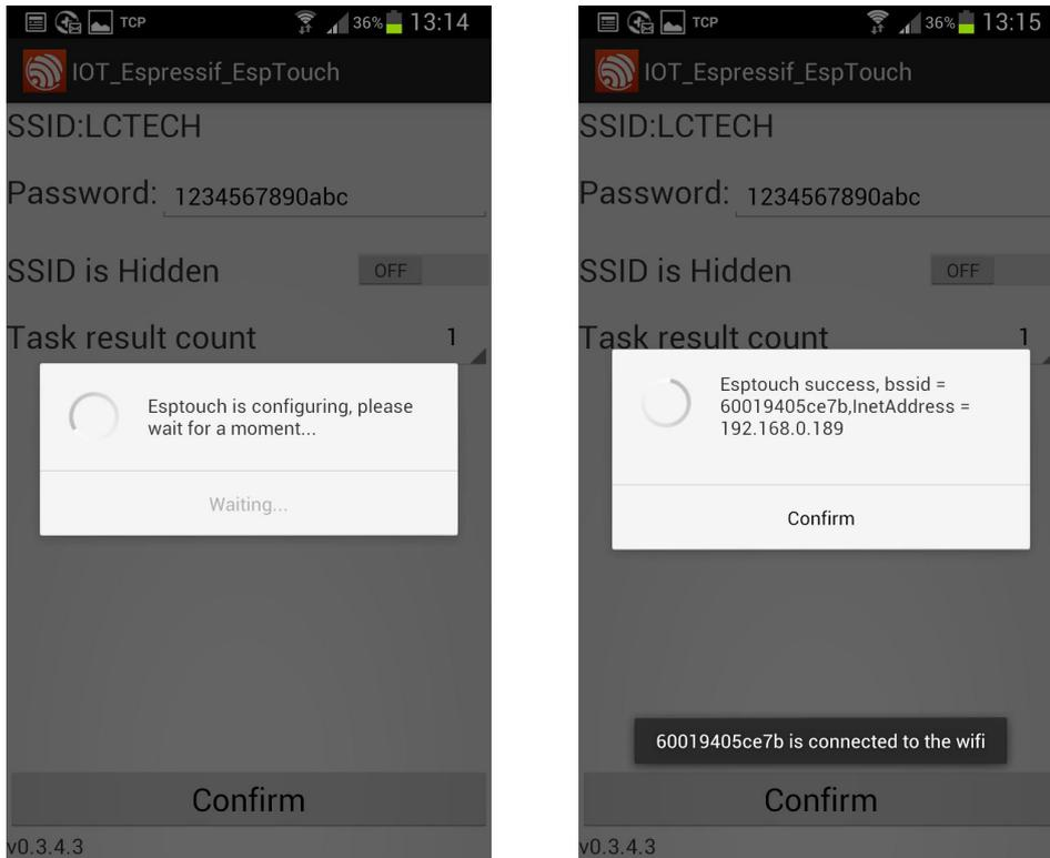
it is important to note:192.168.0.189 this IP address is dynamically allocated by the router to ESP - 01 module.It may change after the next re-connection. User can see the router device list of real-time IP address
