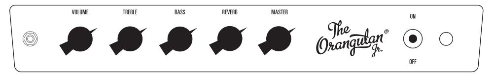
This little guy has two cathode biased 6V6 power tubes and three 12AX7 preamp tubes. Controls are VOLUME, TREBLE, BASS, REVERB, and MASTER. It also has a foot switchable BOOST (which bypasses the bass control, similar to the LIFT on The Orangutan).
