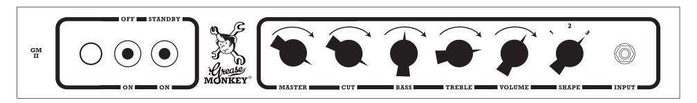
The GM II is an unbridled four EL84 amp with a distinct British voice featuring a switchable HI/LO INPUT GAIN and a MASTER volume control. The BASS and TREBLE controls are extremely interactive and act similar to a parametric EQ. The CUT can be used, after setting the tone controls, to further shape the high end (if needed).
