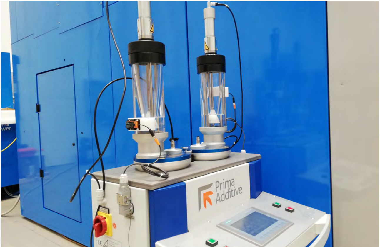
A modular powder feeder suitable for rapid change of material processed or for back-up to increase powder reserve
