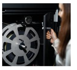
The sealed filament chamber stores two filament spools in an environment shielded from external influences. Drying cartridges further minimize humidity, allowing sensitive materials to be stored at a consistent dryness level.
