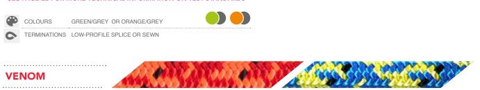
Venom is a lightweight 11.8mm arborist climbing line designed for the new generation of mechanical climbing devices and modern climbing techniques, either on single or doubled rope. Venom has a braided nylon core that works with the 24-plait jacket to give a rope with exceptional flexibility and handling without compromising durability.
