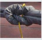
Cow hitch connection, shown with pigtails to assist in separating the connection.
