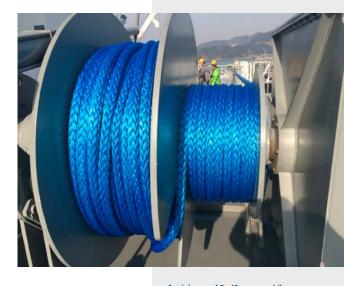
A minimum of 8–10 wraps, while never exceeding one full layer on the tension side of the split-drum, should be maintained at all times while lines are under tension.
