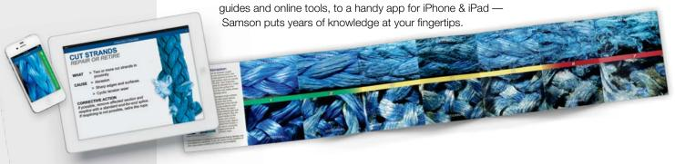
Samson offers a range of tools to assist in inspecting high-performance synthetic lines.
