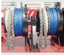
It is important to choose a mooring pendant that provides adequate elongation to reduce dynamic loads induced on the primary mooring lines, especially in exposed mooring berths.
