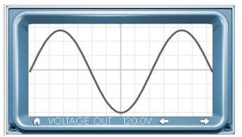
Upon selecting SCOPE the user will first see an oscilloscopic representation of the incoming AC waveform. The image to your left is a visual interpretation of the AC's frequency and distortion, thereby denoting the quality of the power in the home. This is what your components would be receiving if not for the Power Plant 5. Often times the incoming waveform will exhibit a truncated, or chopped-off peak.
