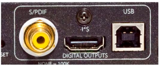
into one stream and then unravelling this compressed format back to I<sup>2</sup>S (as is required for it to work) is typically where jitter is introduced. I<sup>2</sup>S should be the transmission medium of choice if you have a compatible receiver to accept it.
