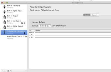
Next you will need to set the sample rate you wish the NPC to operate at. The computer is now the master, the NPC the slave, and will control the NPC when USB is enabled.
