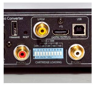
With all the switches down, the cartridge loading is quite high at 100K Ohms. To set the load, simply push the appropriate switches to the up position. The switches must be moved in pairs (one for the left and one for the right channel). For Moving Magnet cartridges, the typical load will be 47K. Move switches 1 and 2 up, keeping the other switches (3-10) in the down position. For a moving coil
