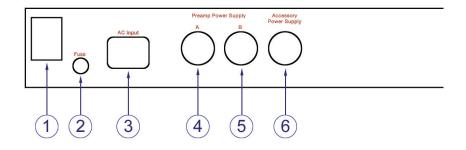
The power switch will illuminate when there is power supplied to the unit and the switch is set to on. The [I] position indicates ON. The [O] position indicates OFF.
