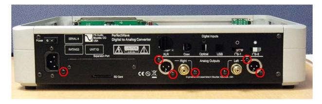
24. Remove AC inlet and ground Faston connectors as shown. A pair of pliers will help with this step. Do not pull on the wires, only the connector. If a PS Bridge is present, remove it at this time.
