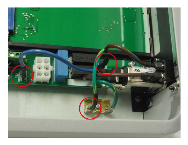
Some PerfectWave DAC (PWD) configurations will require a couple of extra steps in the upgrade process. If your PWD does not have a ground distribution block by the AC inlet, or has a vertical metal wall between the power supply board and the audio boards, then perform the following steps:
