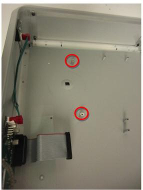
2. Install the new felt pad over the transformer hole.
