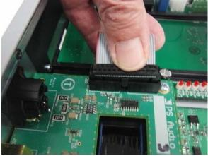
b. Install the new power supply cable between the Power Supply board and the DSD Analog board, and the new ribbon cable between the DSD Digital board and the DSD Analog board.
