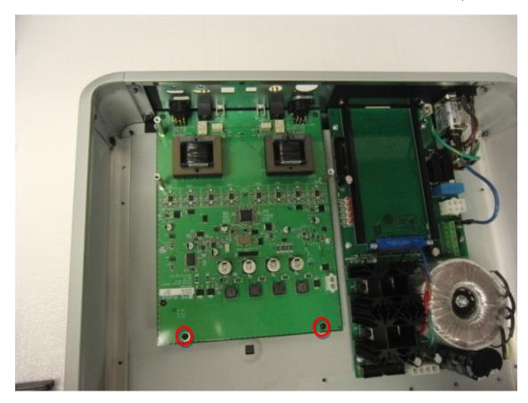
e. Insert 3 each #6-32 X 1-1/4" hex male-female spacer into the three holes closest to the rear panel. Finger tight only, no wrenches.
