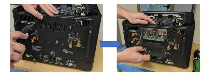
CAUTION/WARNING: BEFORE PROCEEDING FURTHER: the RED LED in the tube compartment must be off. If the LED is lit, wait for it to go out. The LED when lit indicates the presence of high voltage.
