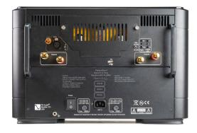
• Ground Binding Post: On the lower left of the back panel is a grounding post with a "Ground" symbol. Few of you will ever need or use this. It's used only in limited and specific situations, such as for certain powered subwoofers discussed below.
