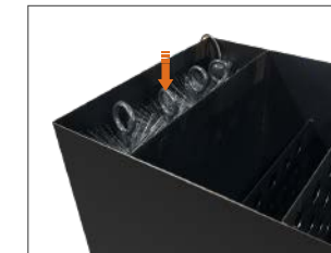
Step 3. 1 layer put in the filter brush and UV lamp.
