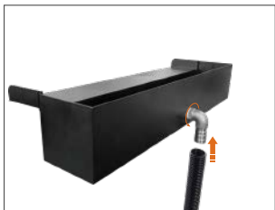
Step 2. Attach the pond tube to the waterfall box.
