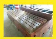
FC25 tough cast iron with quenched treatment MEEHANITE certificated casting to ensure the high rigidity and greater accuracy, heat treated work bench surface above HRC65.
