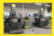
Custom-made machine: Generator with 4-independent spark channels and 360-degree work tank.
