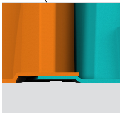
Overlap i bunden imellem Endemodulet og den store ribbe.
