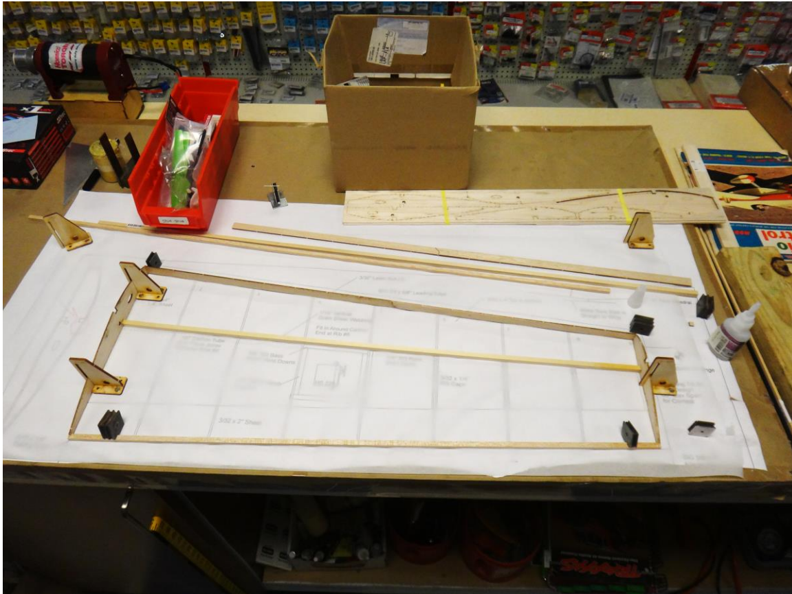
Perimeter layout Wing-It stock shape for my V tailed "Victor" design.
