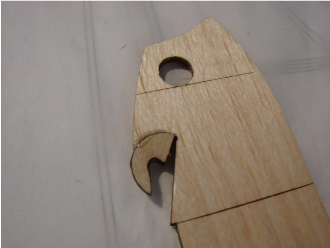
Glue ply piece covering half of the slot.
