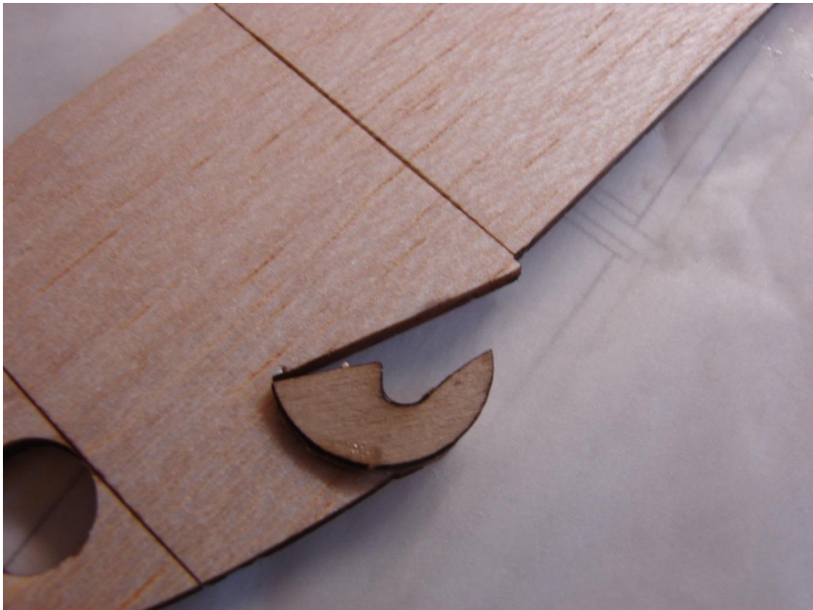
Glue ply piece covering half of the slot.
