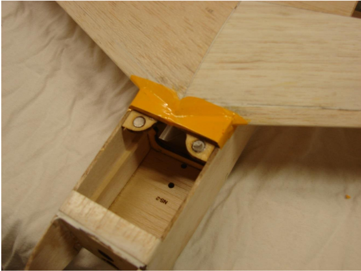
Front cover filler, makes the wing to fuselage covering transition easier.
