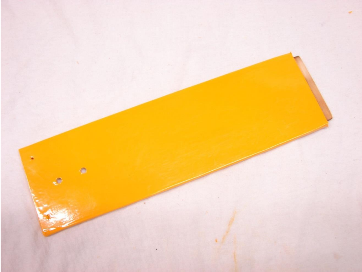
Hatch prepped for screws and Skid.
