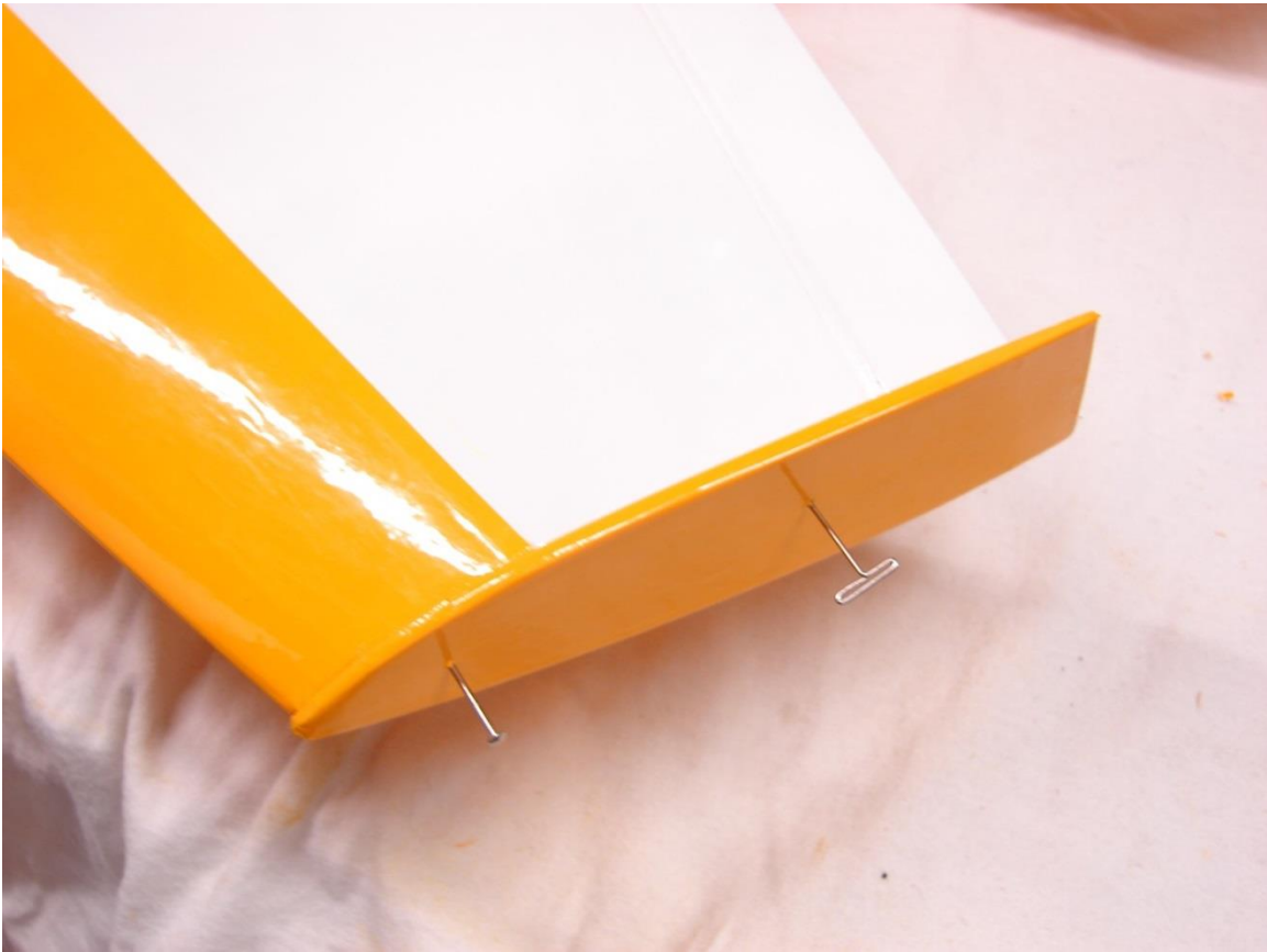
Epoxy on the endplate.
