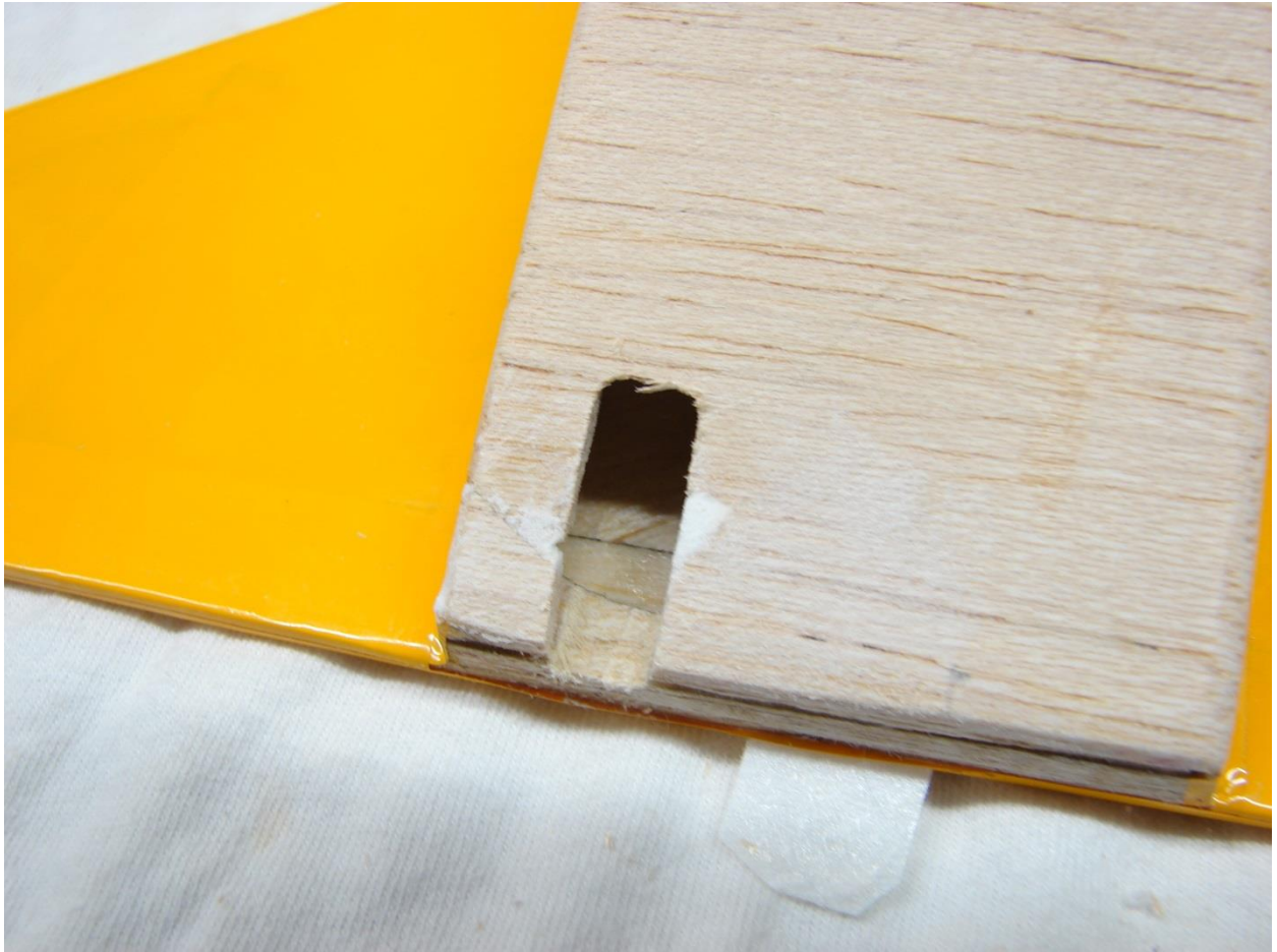
Elevator exit detail.
