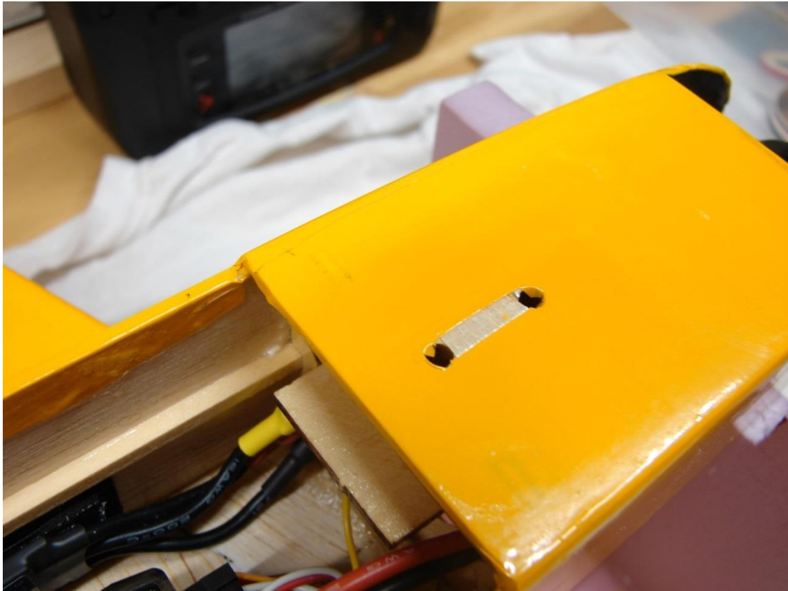
Prepare the fuselage nose for the skid.
