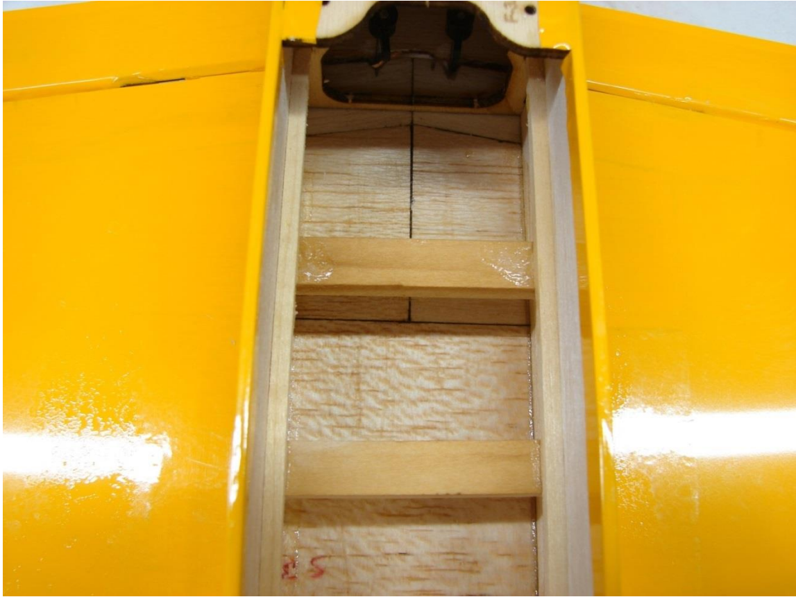
Glue (C) bass servo rails in place.
